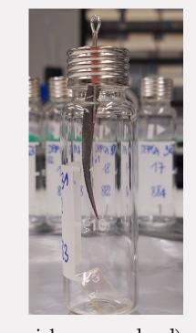
Figure 2. (left) Daily analysis comprising a set of vials (3 replicates x 3 sample type, along with a standard); (center) PDMS-HLB membrane; (right) containment unit ready for headspace sampling.
