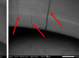
Images above: All the rings, including the control, presented new or expanded cracks following the second examination under SEM.
