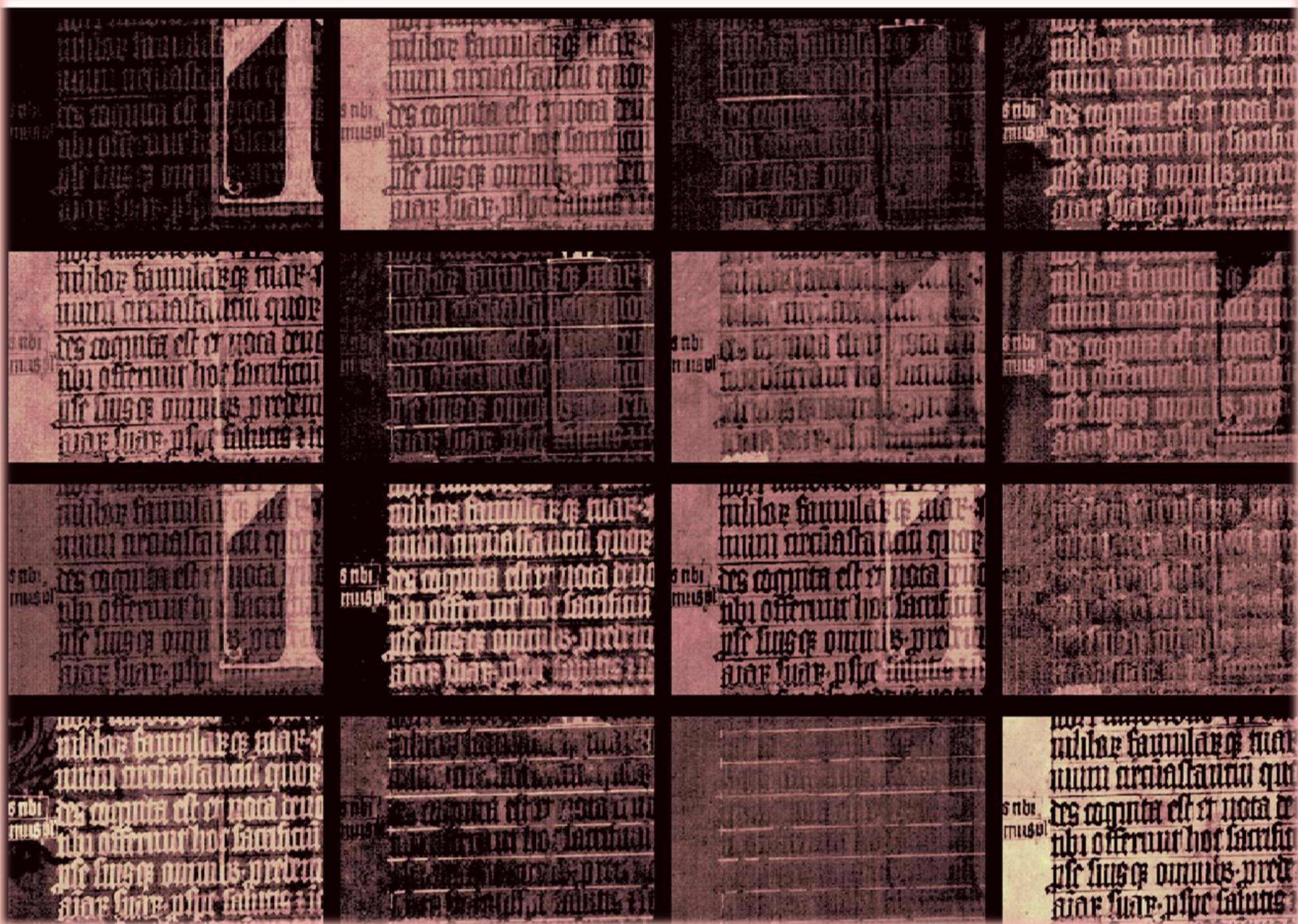
Figure 1: Fusion Image Cube Abundance Maps of a Kepler volume manuscript bound cover held by UCL Special Collections; STRONG ROOM C 1606 K2/2. HSI-XRF Co-Registered, source-level fused. Endmember estimation through NWHFC. Endmember extraction using NFINDR identified 16 endmembers. LMM abundance maps produced with FCLS and plotted in sequence.
