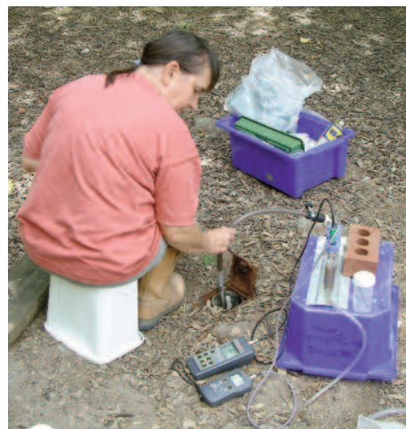
Figure 20 Water level can be measured in a borehole using an audible dip meter. Here Christine Elgy is taking measurements of water temperature, redox potential and pH in Droitwich with portable probes and meters, using flow-through system to reduce contamination. Photo: Worcestershire County Council
