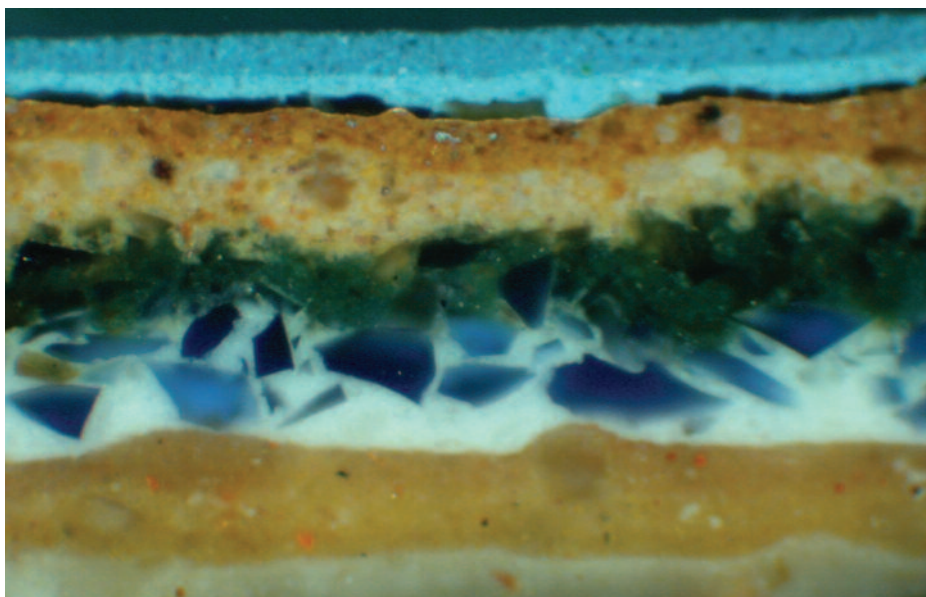
Figure 11 A cross-section of a paint sample taken from the frieze of the Star Chamber, Bolsover Castle. Image courtesy of Helen Hughes. © English Heritage.
