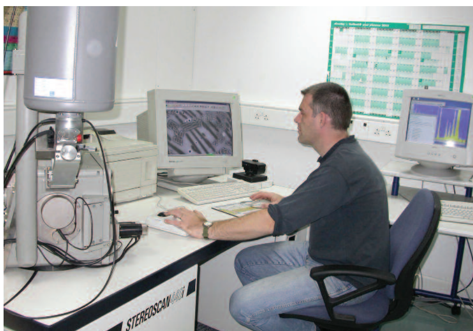
Figure 7 SEM examination and EDS analysis of copper alloy slag from a 17th-century context in Colchester. The analysis showed that the alloy used was of the sort used in the manufacture of cauldrons (not bells). © English Heritage.
