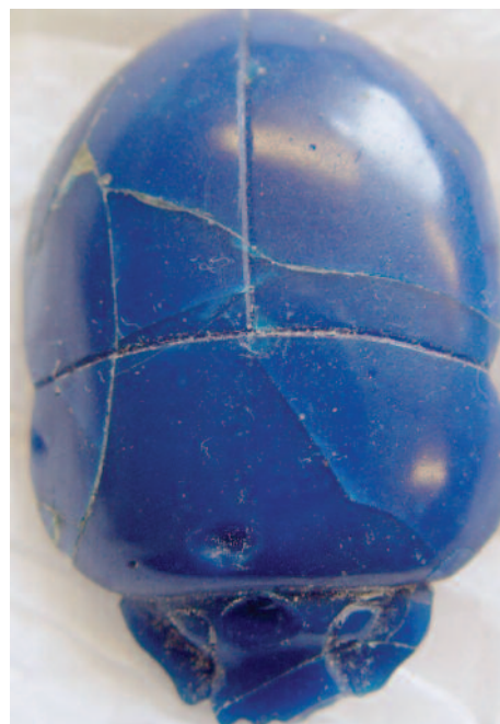
Figure 14 An Egyptian glass scarab from the British Museum. Compositional analysis of the glass aided comparison with other similar items, dating the object to the Third Intermediate Period. However, the analysis also provided vital information about why the object was degrading, enabling recommendations to be produced for its future storage. © Trustees of the British Museum.
