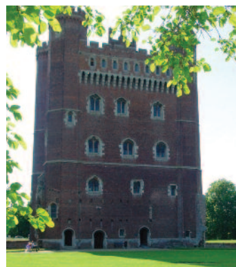
Figure 10 Luminescence dating of known age buildings, such as Tattershall Castle, Lincolnshire (shown here), to assist in the development of this technique. The independent date range for the sampled part of the building was AD1445-1450, luminescence dates were 1455 \pm 33 and 1455 \pm 34 . Image and data courtesy of Ian Bailliff.
