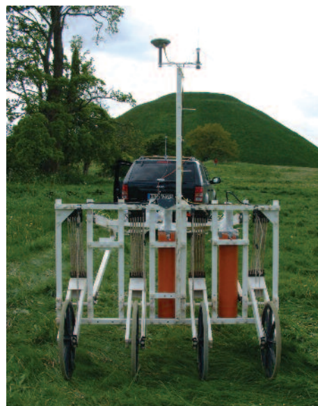
Figure 8 Towed magnetometer array consisting of two SQUID gradiometers with integral GPS system. Photo courtesy of Neil Linford. © English Heritage.
